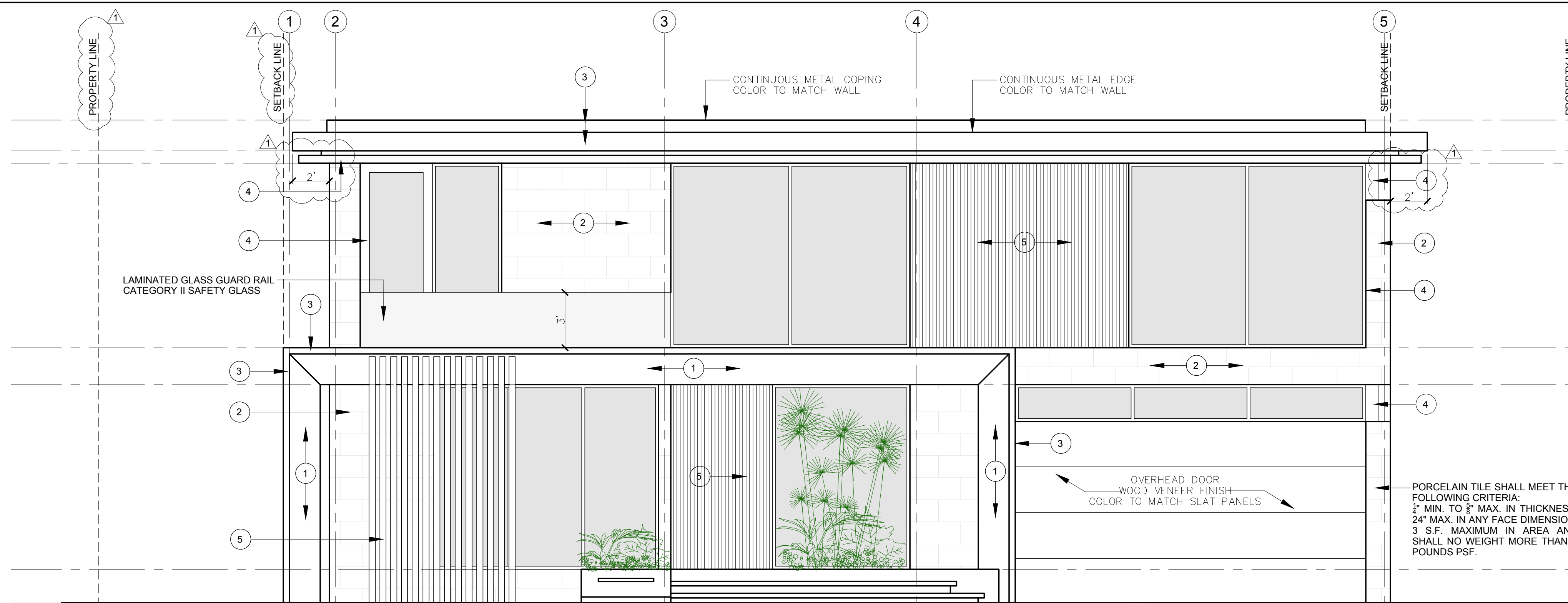
1 FRONT (NORTH) ELEVATION A-2.0 1/4" = 1'0"
