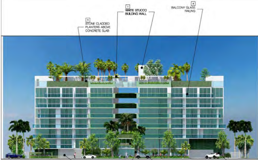
NORTH ELEVATION [FRONT]
