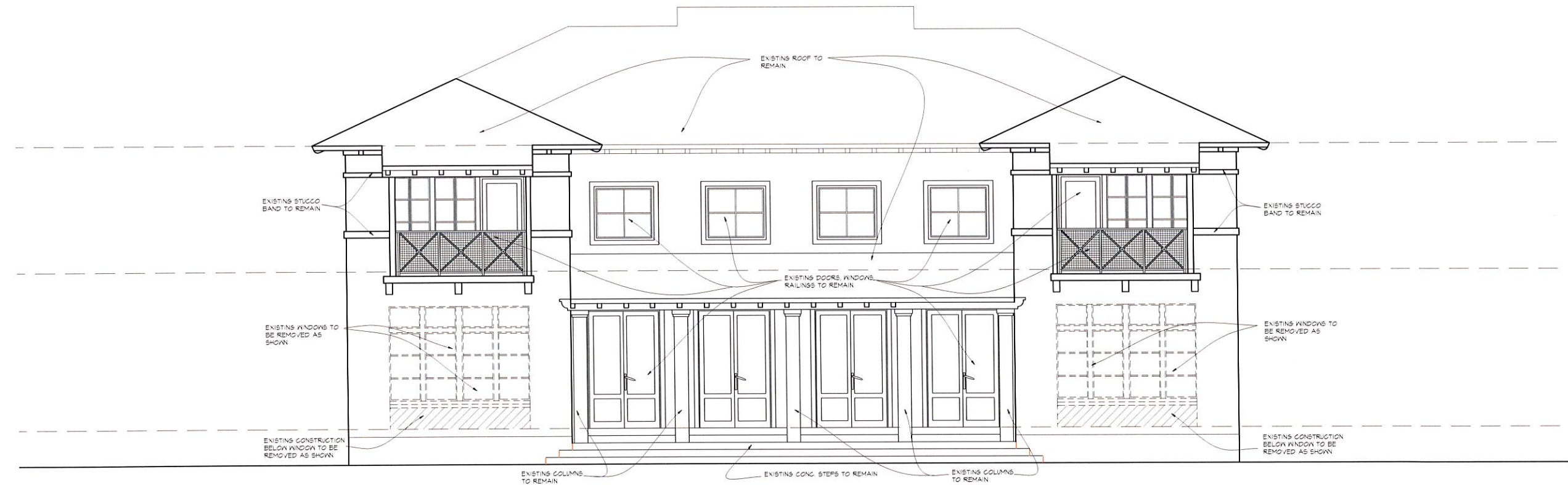
DEMOLITION REAR ELEVATION SCALE: 1/4"=1'-0"
