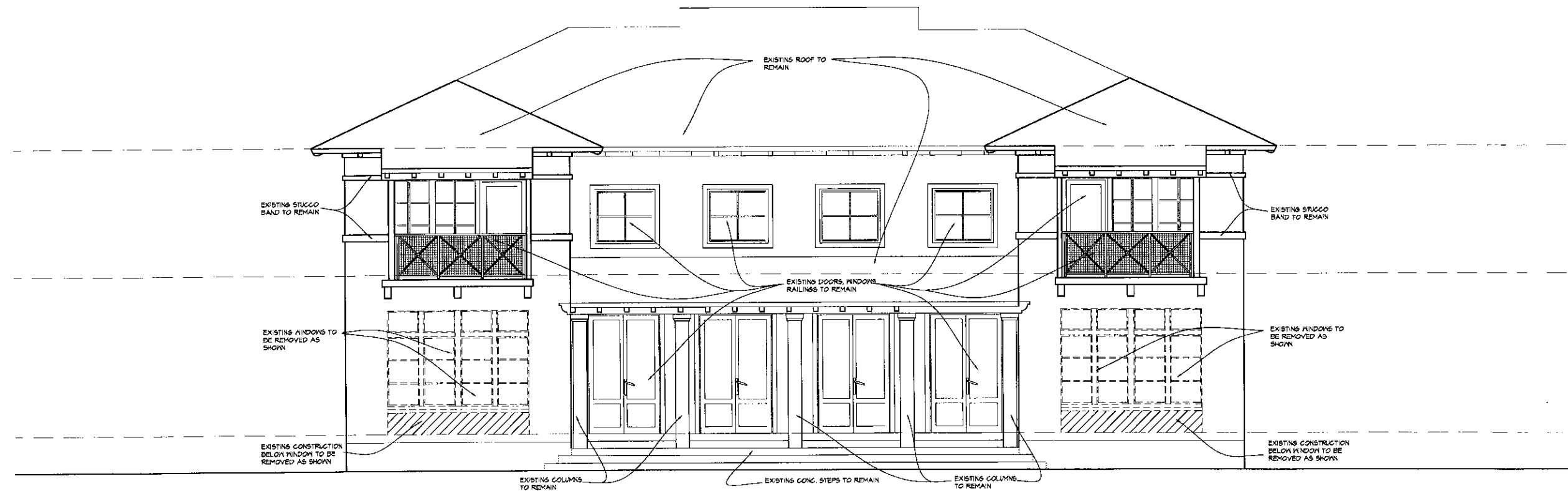
DEMOLITION REAR ELEVATION SCALE: 1/4"=1'-0"
