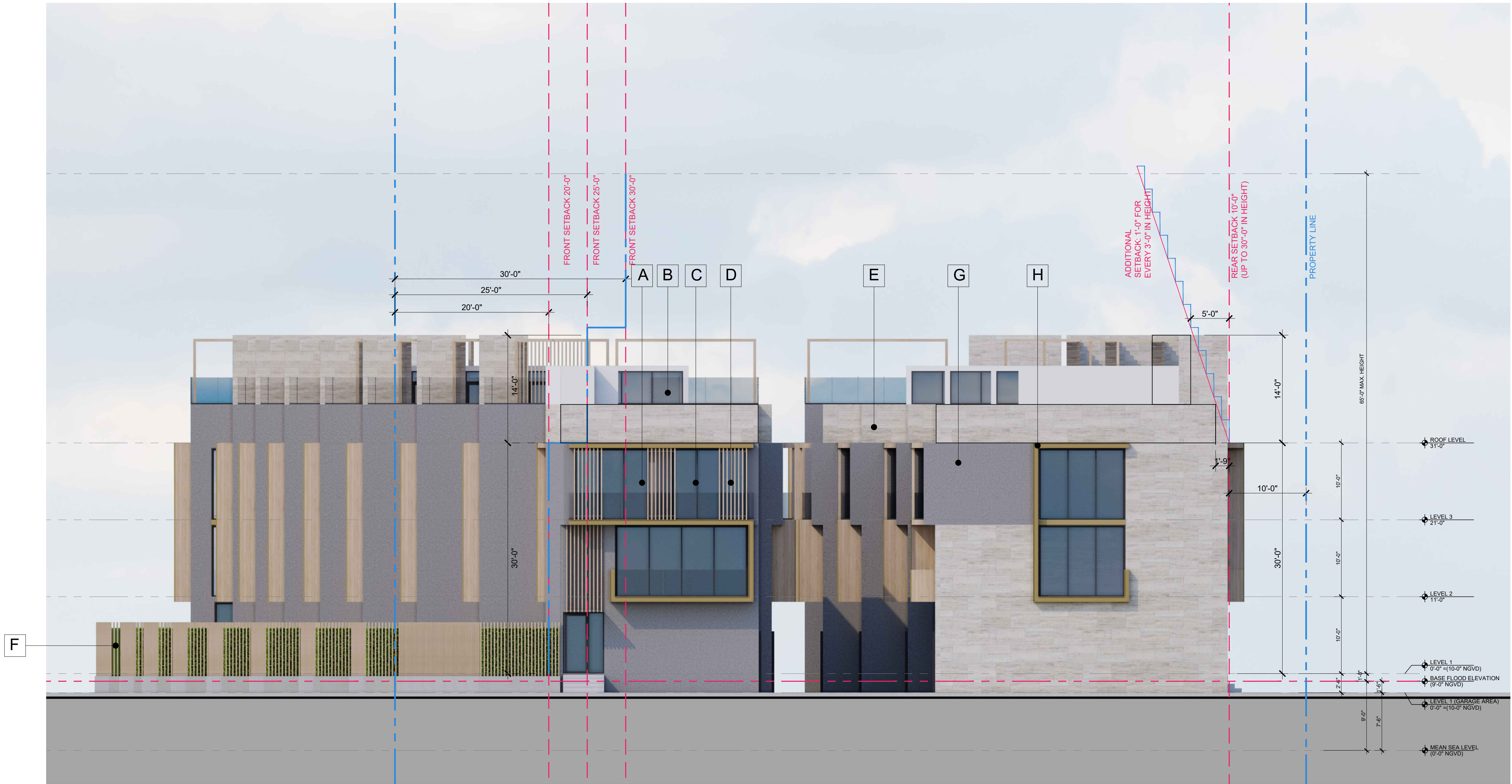
3 BUILDING ELEVATION - NORTH SCALE: 1/8" = 1'-0"
