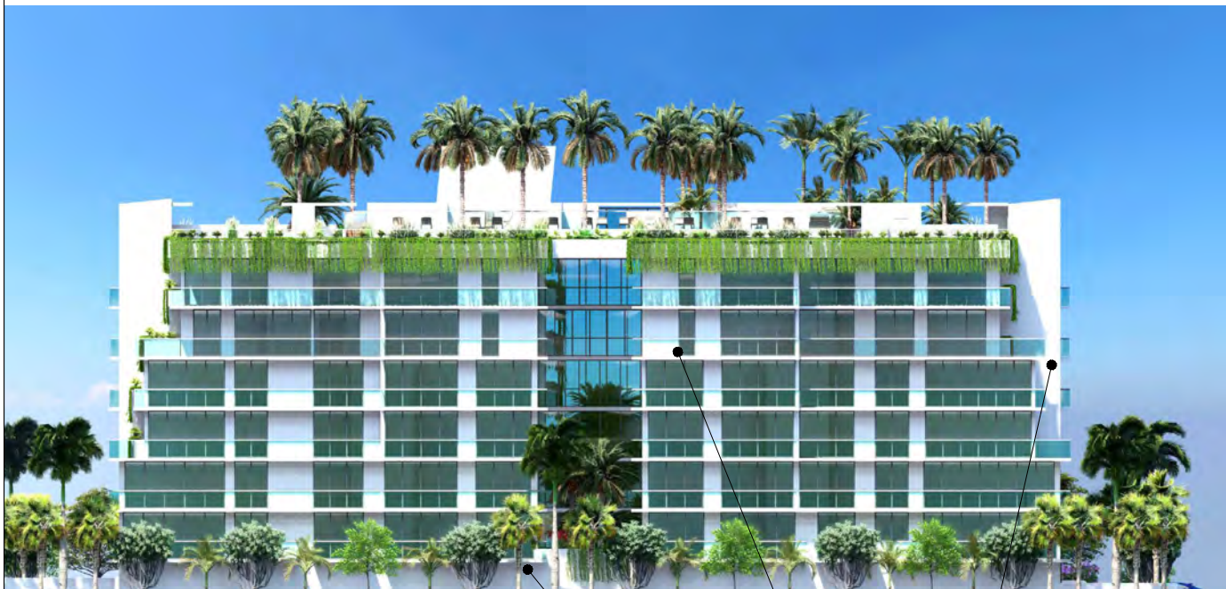
NORTH ELEVATION [RIGHT SIDE] 2 GRAY ALUMINUM GARAGE LOUVERS 4 GLASS BALCONY RAILING 4 WHITE STUCCO BUILDING WALL SOUTH ELEVATION [LEFT SIDE] 2 GRAY ALUMINUM GARAGE LOUVERS 4 GLASS BALCONY RAILING 4 WHITE STUCCO BUILDING WALL
