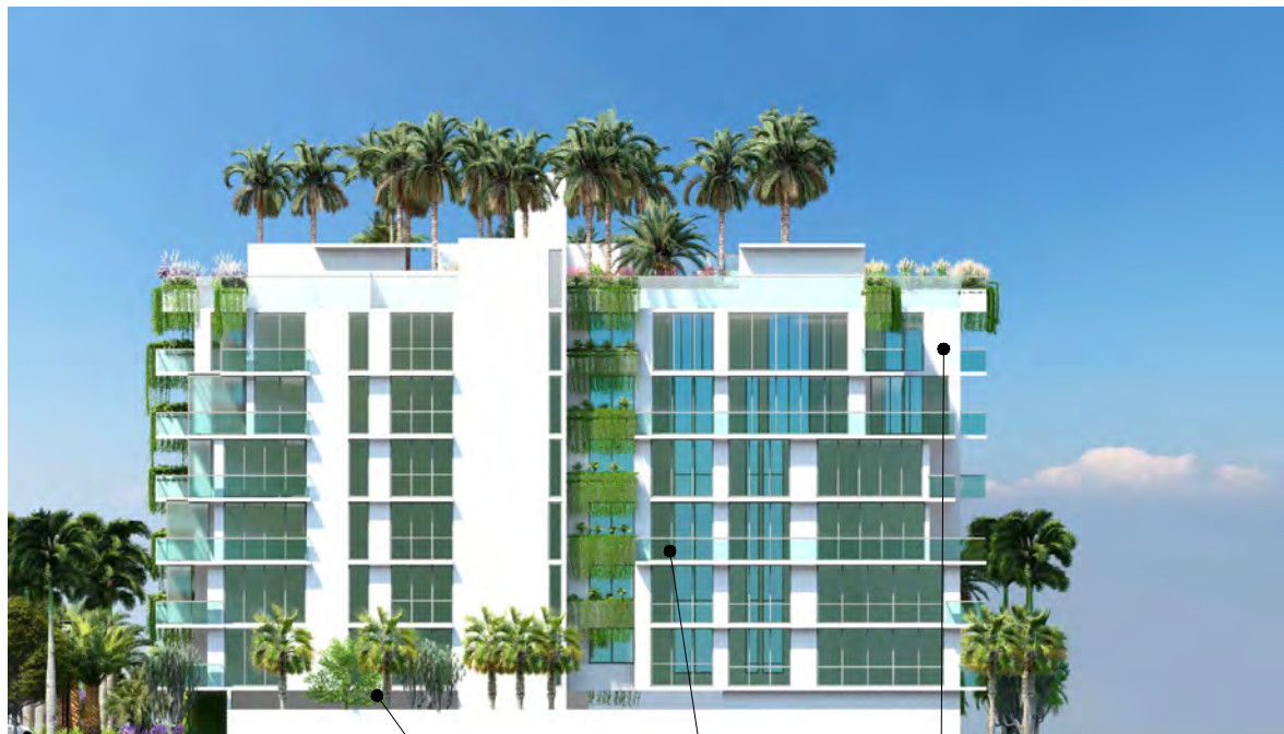
NORTH ELEVATION [RIGHT SIDE] 2 GRAY ALUMINUM GARAGE LOUVERS 4 GLASS BALCONY RAILING 4 WHITE STUCCO BUILDING WALL SOUTH ELEVATION [LEFT SIDE] 2 GRAY ALUMINUM GARAGE LOUVERS 4 GLASS BALCONY RAILING 4 WHITE STUCCO BUILDING WALL
