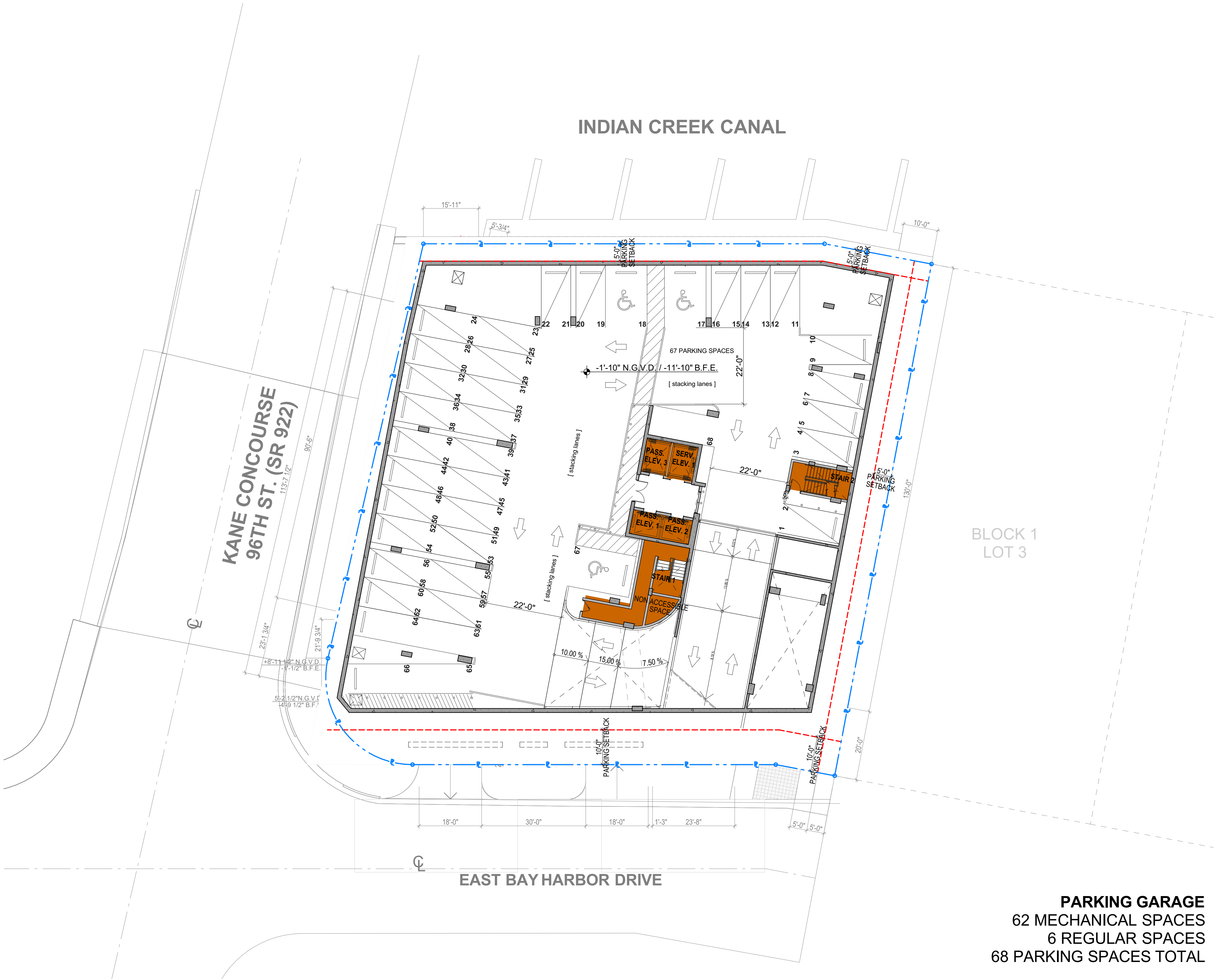
1 BASEMENT PARKING -1 SCALE: 1/16" = 1'-0"
