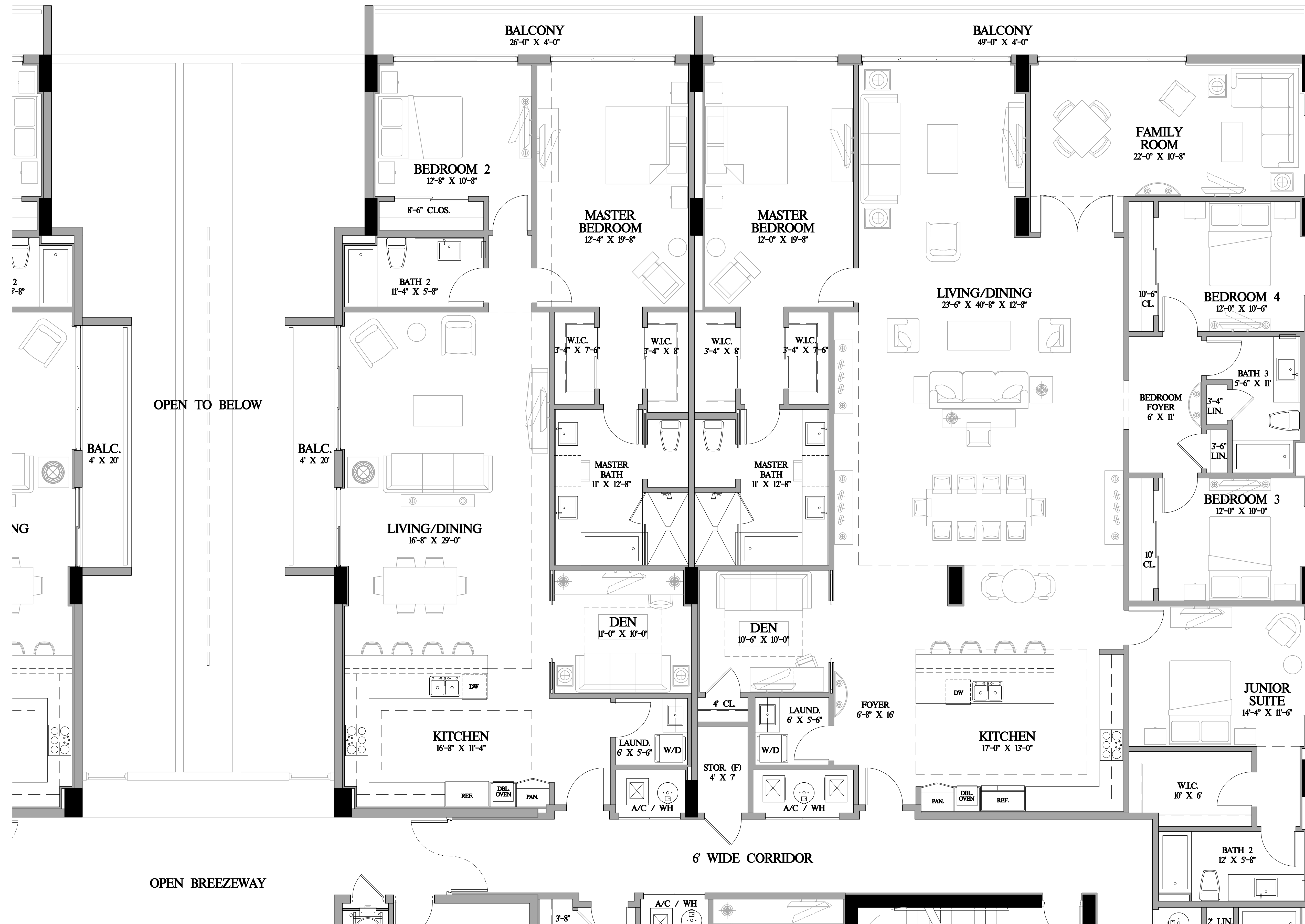
LEVEL 3 - NORTHEAST UNIT FLOOR PLANS SCALE: 1/4" = 1'-0"
