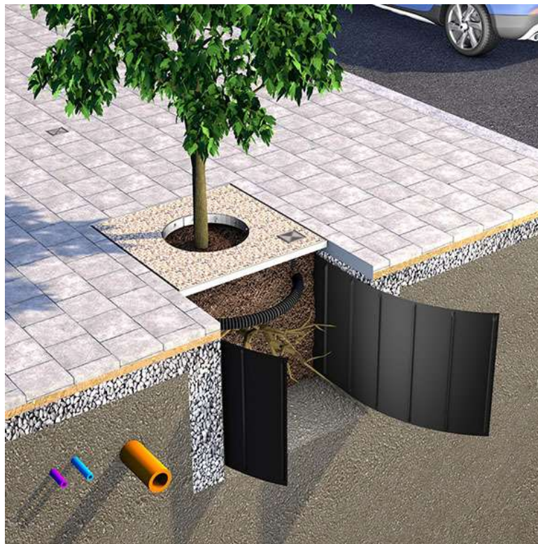
Figure 2: Root Barriers near Brick Pavers
