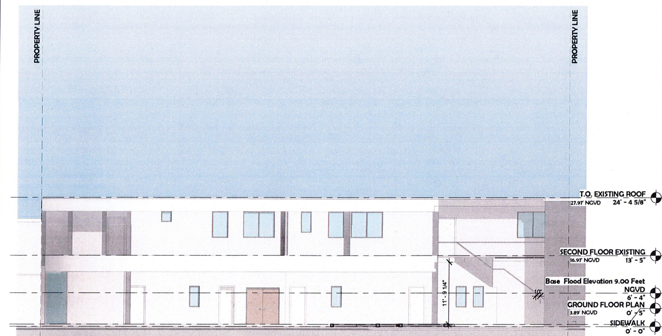
1 EXISTING NORTH ELEVATION 1/8" = 1'-0"
