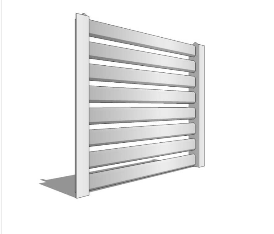
ALUMINUM SCREEN FOR MECH. & POOL EQUIPMENT
