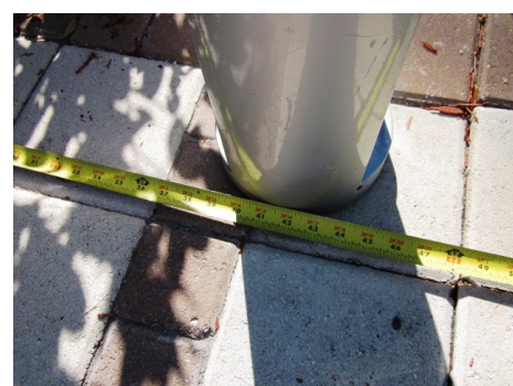
North gate offset pull side 12 inches
