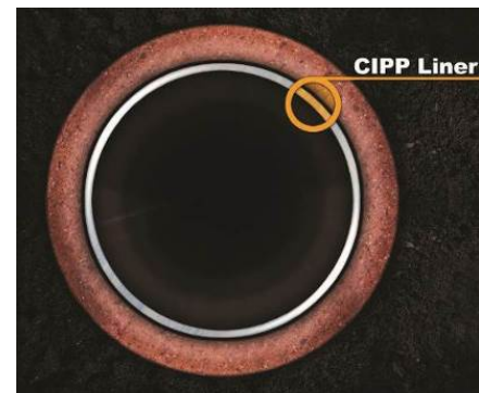
Fig 1. Trenchless CIPP Lining
