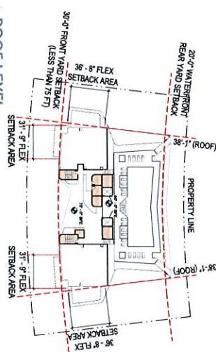
ROOF LEVEL SCALE: 1" = 40'-0"
