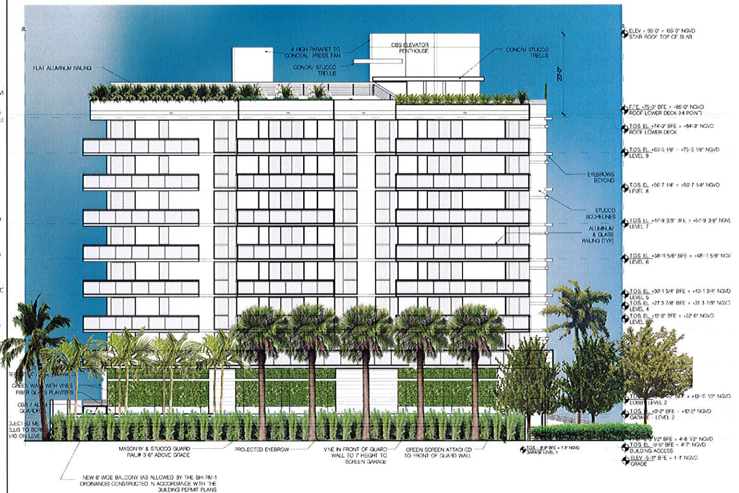
NORTH ELEVATION - REVISED FOR CONSTRUCTION SCALE : 3/32" = 1'-0"
